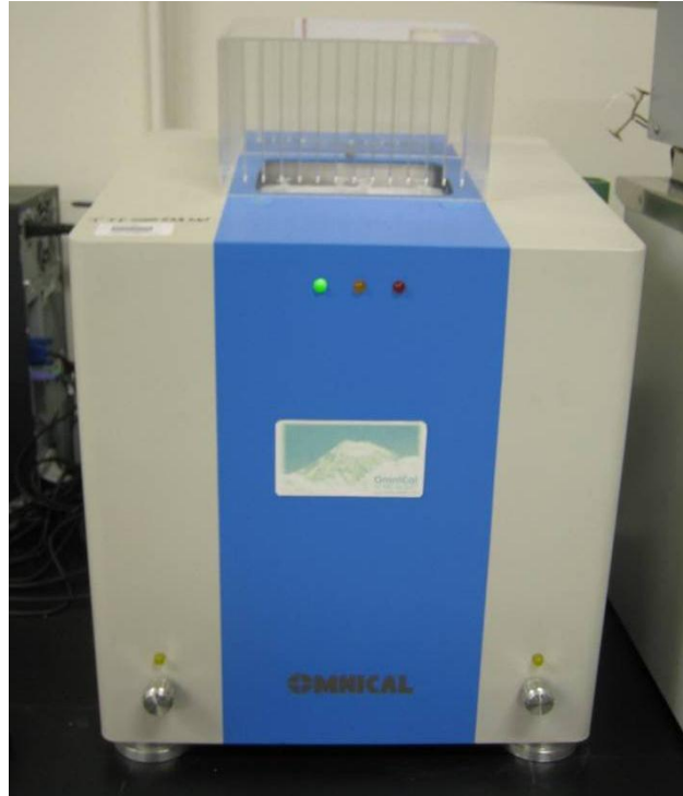
Figure 4-5 Isothermal conduction calorimeter for the heat of hydration of cement paste.
