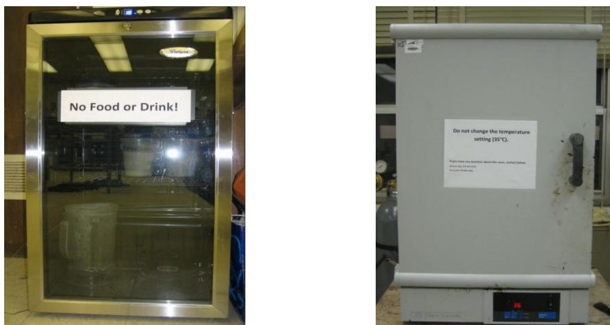
Figure 4-1 Use of the refrigerator to mix at low temperature (left) and the oven to mix at high temperature (right).
