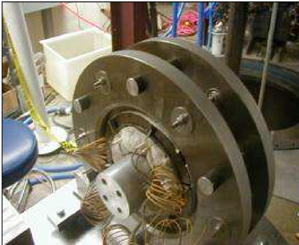
Figure 3-12 Stator with support rings and dummy shaft
