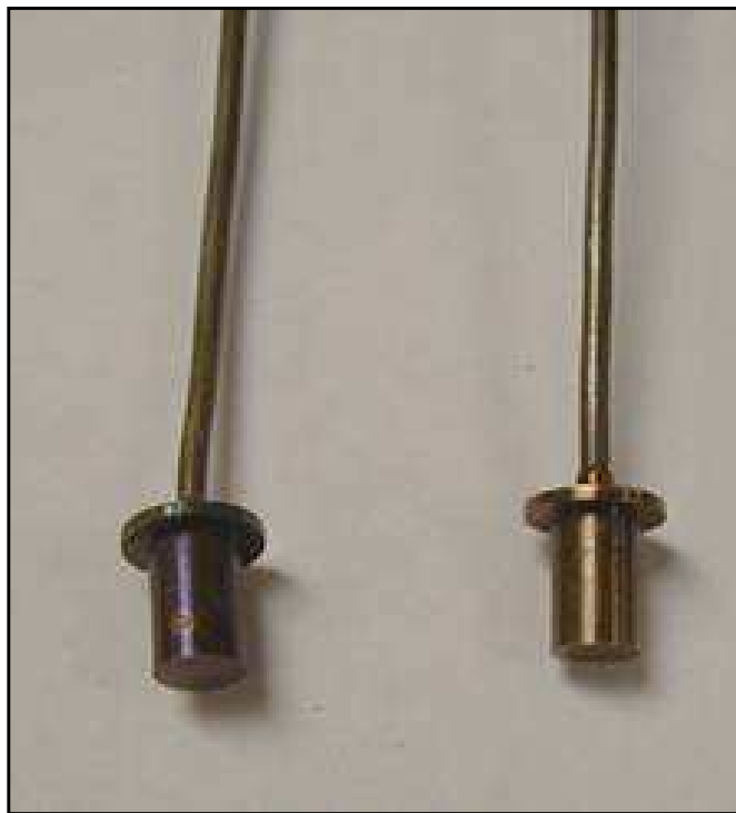
Figure 5-18 High temperature sensors after and before heat test
