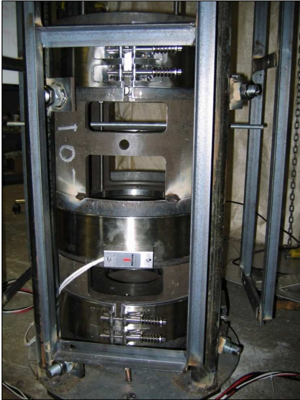
Figure 6-8 Band heater mounted on the outer cylinder
