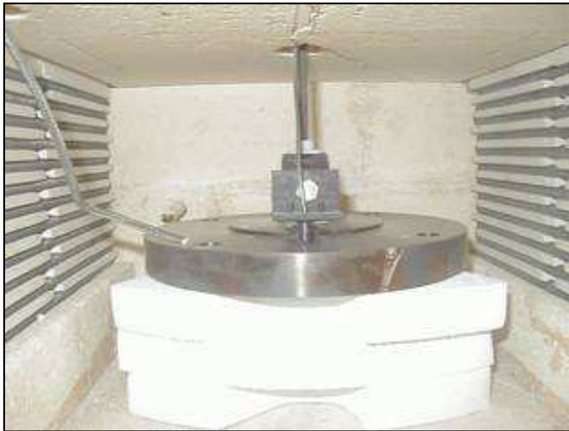
Figure 5-17 Clamping mechanism for sensor
