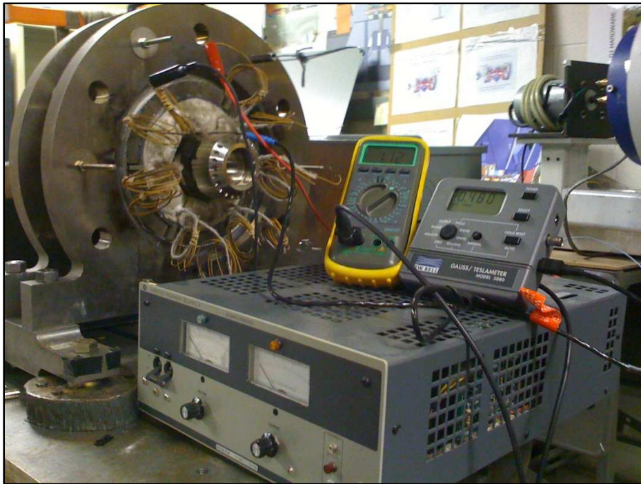
Figure 4-7 Test setup to measure control flux density
