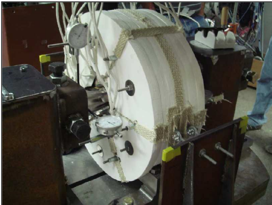
Figure 3-19 Zircar insulation on the rig
