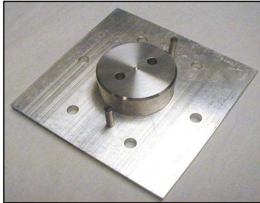
Figure 3-8 Fixture for laminate alignment
