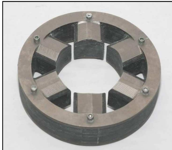
Figure 3-9 Stator made using laminates
