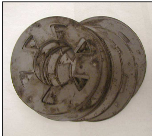
Figure 3-7 Hiperco-50 stator laminates
