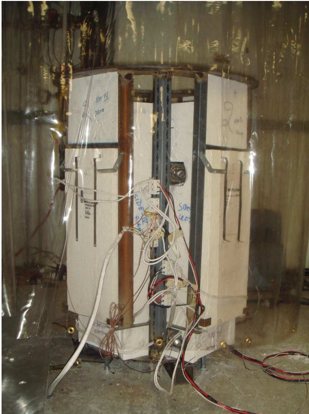
Figure 6-10 Zircar insulation and radiant heaters mounted
