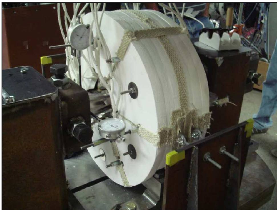
Figure 3-1 Radial bearing force test rig
