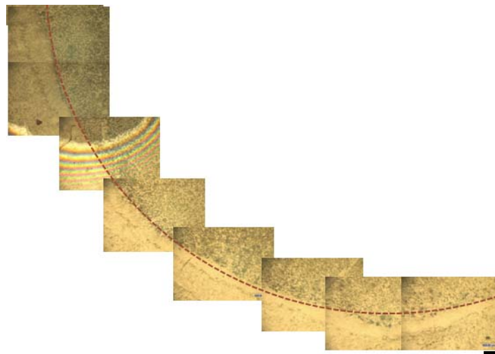
Figure 27 R c =1.158cm for S15_10. With VHX-600 Keyence microscope. The scale bar indicates 500 \mu m.
