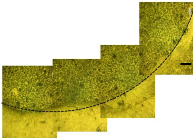
Figure 30 R_c=0.631\text{cm} for S19_55. With VHX-600 Keyence microscope. The scale bar indicates 500\mu\text{m} .
