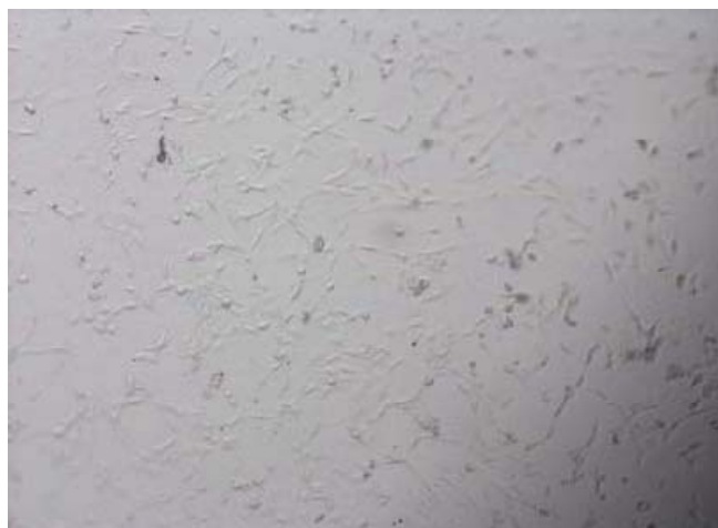
Figure 13 3T3 mouse fibroblasts at 3 days of culture on 2, 6 Bis(3 amino phenoxybenzo nitrile) ( \beta -CN APB) at 10X magnification with an Axiovert A200 inverted transmission microscope (Carl Zeiss).
