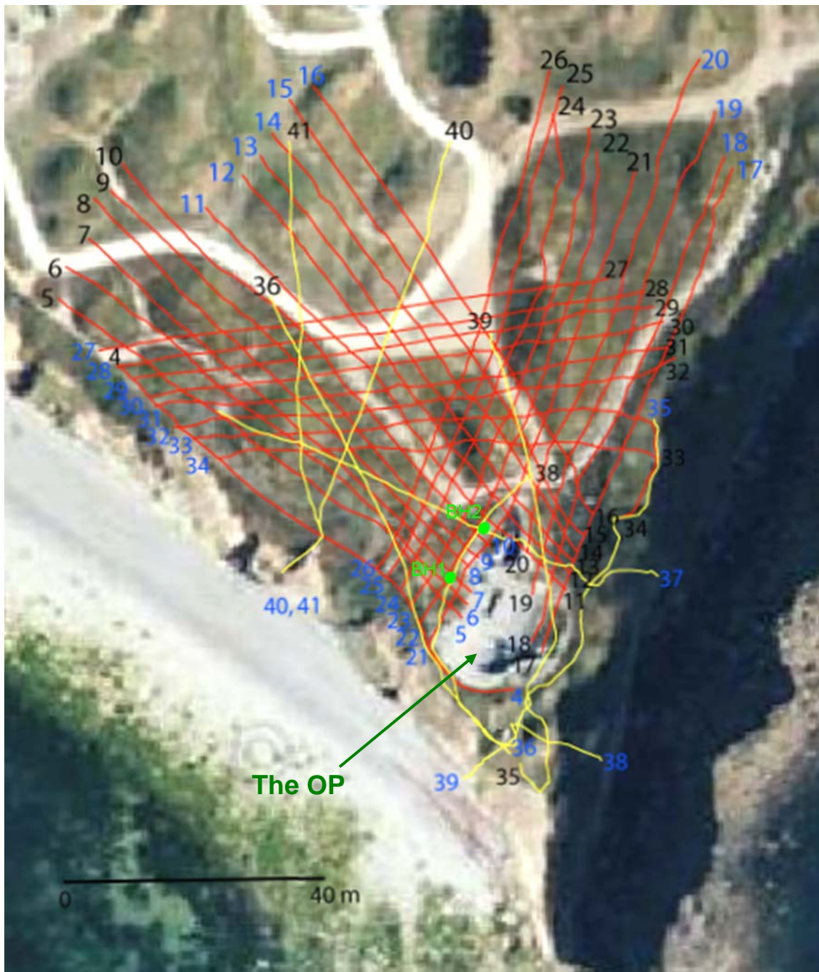
Figure 4.6. Pointe du Hoc 2008 OP geophysical site map showing locations of topside resistivity lines (red), cliffside resistivity lines and other lines that required roped access (yellow) at the OP area. Green dots are borehole locations acquired in 2008 by the geotechnical team. The start of each line is marked by the blue numbers, while the end of each line is marked by the black numbers.
