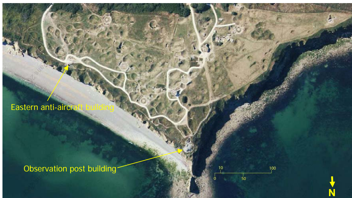
Figure 1.2. An aerial view of the Pointe du Hoc site. Notice the extensive gravel shingle that accumulates on the east side during quiet periods between large storms.
