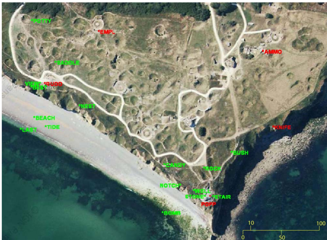
Figure 4.5. Total-station temporary control point network used for locating electrode positions in the 2008 data acquisition phase. Overall site control points are in red while additional control points for the Observation Post and Rudder's Command Post areas are in green.
