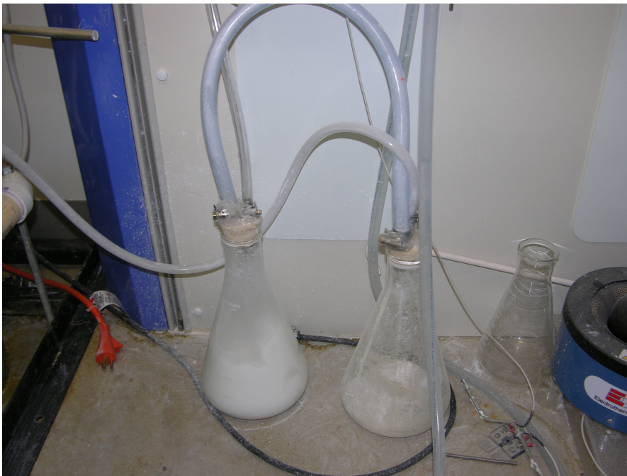
Figure 2-4. Photograph of lime slurry container.
