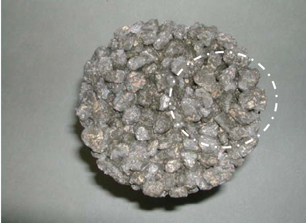
Figure 26 The top of sample incorporating both 9.5 mm and 12.5 mm aggregates. The white circle indicates a region of poor compaction.
