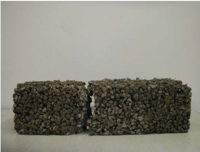
Figure 32 6 in. x 6 in. x 12 in. beam sample after flexural test (polypropylene).
