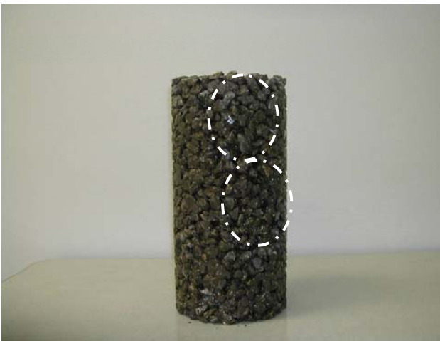
Figure 27 The side of sample incorporating both 9.5 mm and 12.5 mm aggregates. The white circles indicate regions of poor compaction.
