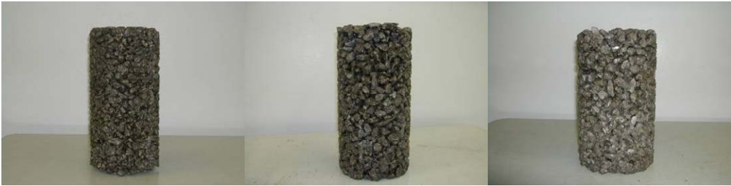
Figure 23 Picture of samples (from left to right, low coarse aggregate, mid coarse aggregate, and high coarse aggregate).
