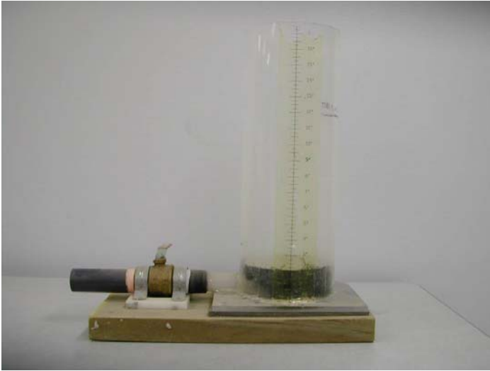
Figure 39 Device used to clog pervious concrete cylinders using sand/water mixture.
