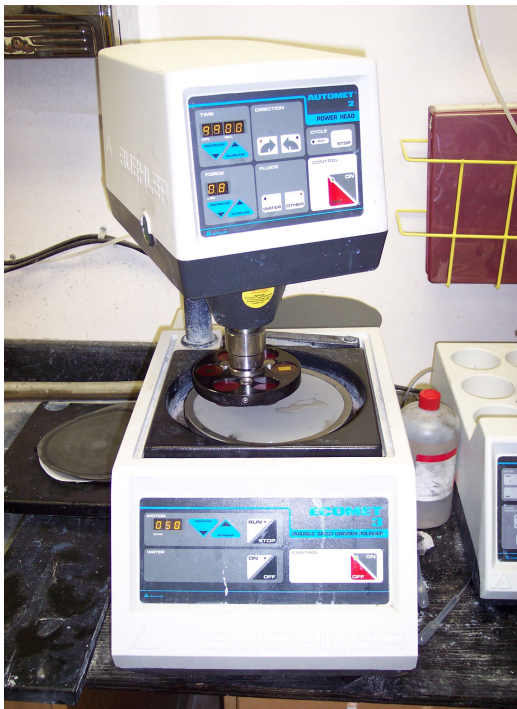
Figure 17. Autopolisher for sample preparation.
