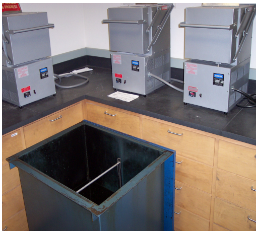
Figure 14. Arrangement of furnaces and oil bath.
