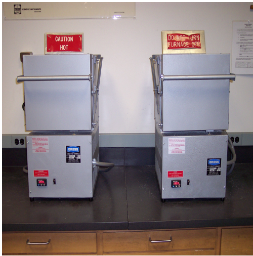
Figure 12. Preheated furnaces for step 1 and 2.
