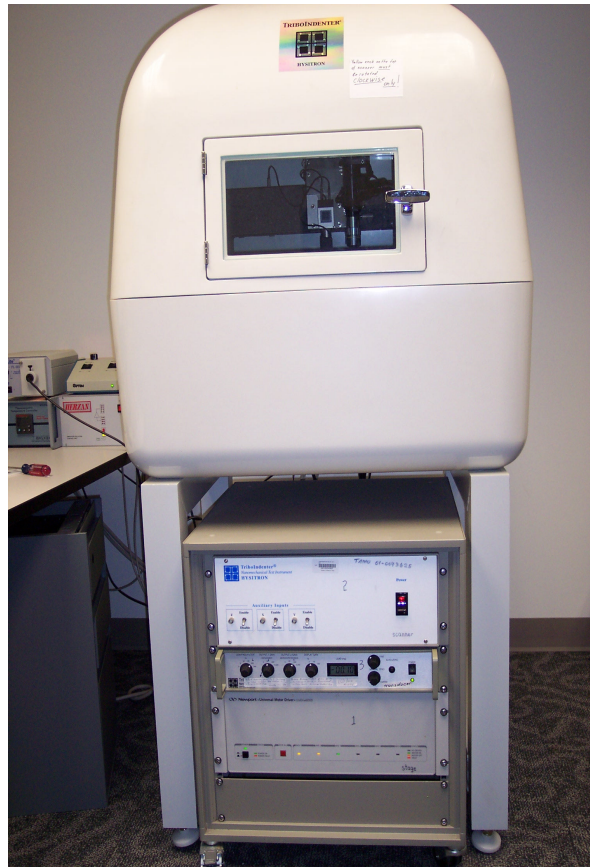
Figure 5. Hysitron's TriboIndenter nanoindenter with environmental cover.
