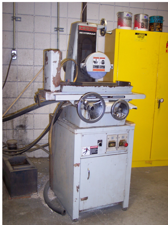
Figure 16. Grinder used to smooth rough-cut samples.
