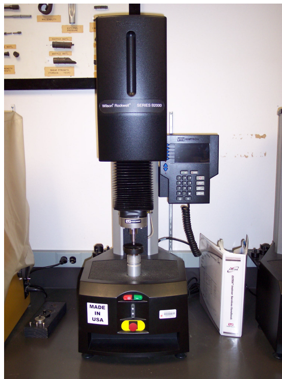
Figure 3. Instron Series 2000 Rockwell® hardness tester with Wilson test block and penetrator.
