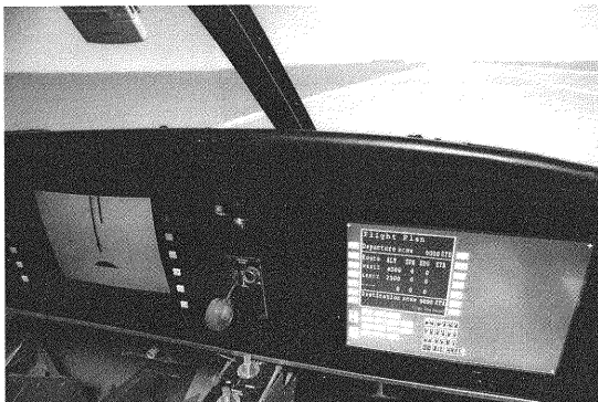
Figure 4.9 Left and Right Head Down Displays of the Engineering Flight Simulator Cockpit
