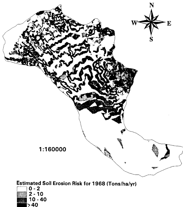
Figure 9. Universal Soil Loss Equation estimates of the soil erosion pattern within the El Pital watershed in 1968
