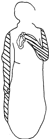
Figure 158. Laminations on the "Joan of Arc" figurehead at Mystic Seaport Museum. (Drawing by Carol Olsen.)
