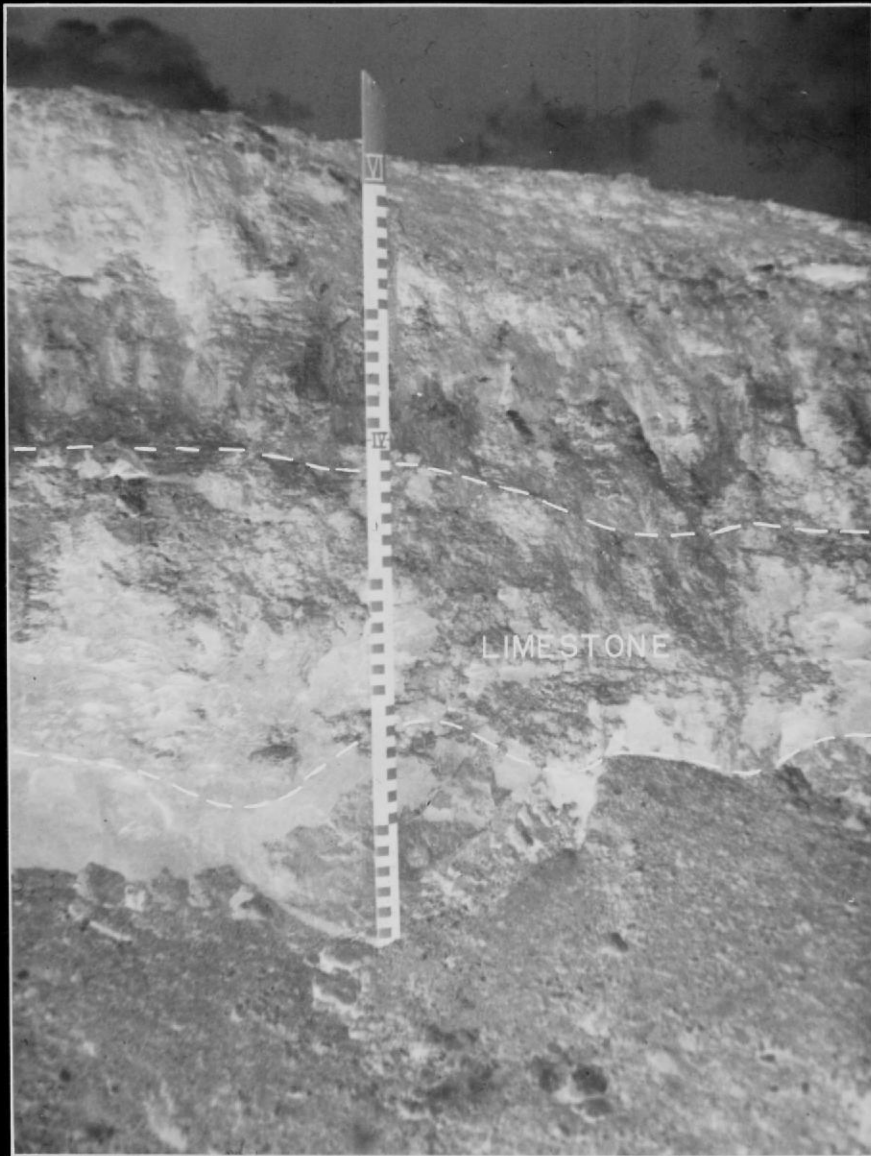
Exposure of white, soft, poorly-bedded caliche and massive layer of medium-gray, sublithographic limestone in the south wall of the caliche quarry on the Nell Harris property about 2.2 miles north of Pontotoc.
