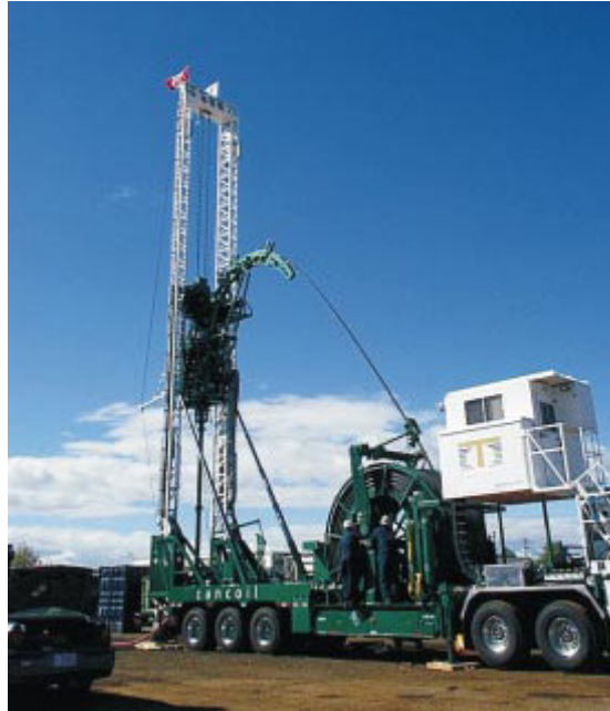
Fig. 3.8 — Typical coiled tubing rigs 60
