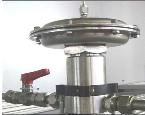
Fig. 4.14- Tescom backpressure regulator.
