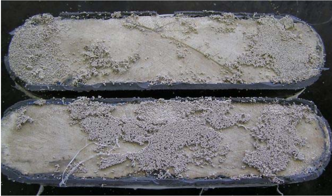
Fig. 4.3- Proppant placement of Experiment A.
