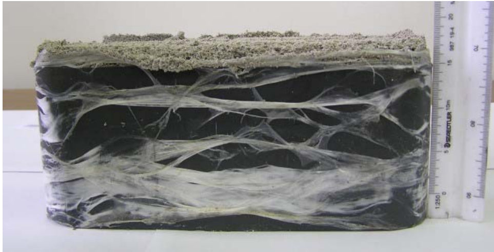
Fig. 4.11- A screen out experiment.
