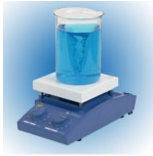
Fig. 4.7- A magnetic stirrer and a created vortex.
