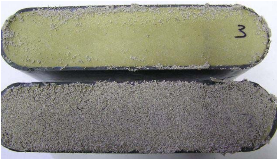
Fig. 4.6- Proppant placement of Experiment B.
