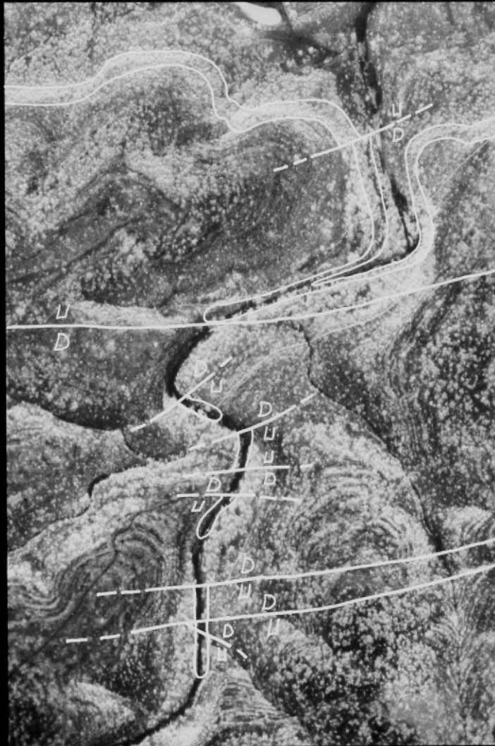
Aerial photograph showing repetition of the Welge outcrops due to faulting. (Welge outcrops are marked with light lines and the faults are marked with heavy lines.)
