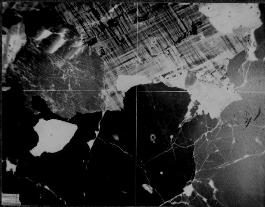
Photomicrograph of fine-grained granite, showing some of the primary minerals (crossed nicols, x20)
