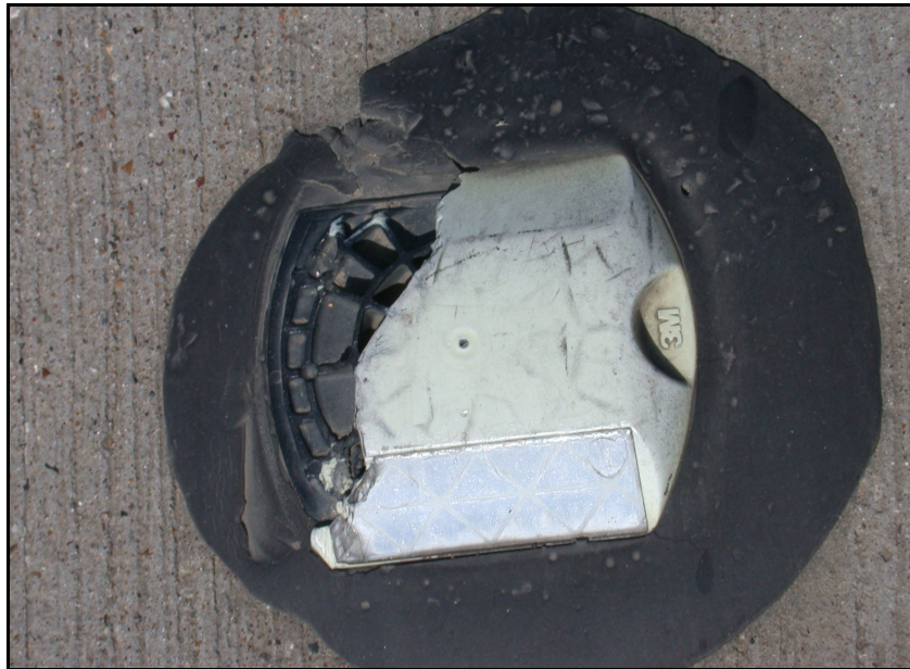
FIGURE 10 Damage at the non-lens side of a RRPM.
