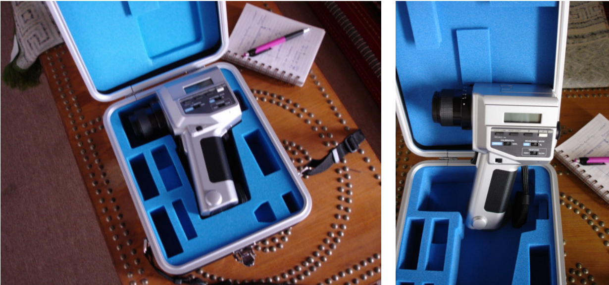
Fig. 16 Luminance meter Konica Minolta LS-110
