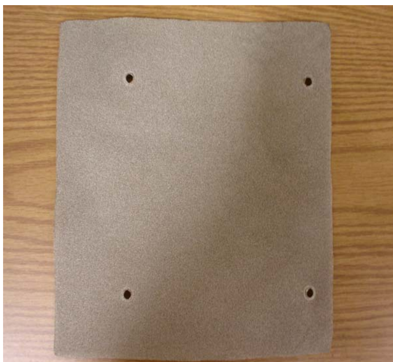
Figure 11: Ni-metal foam flow field used in this research project.
