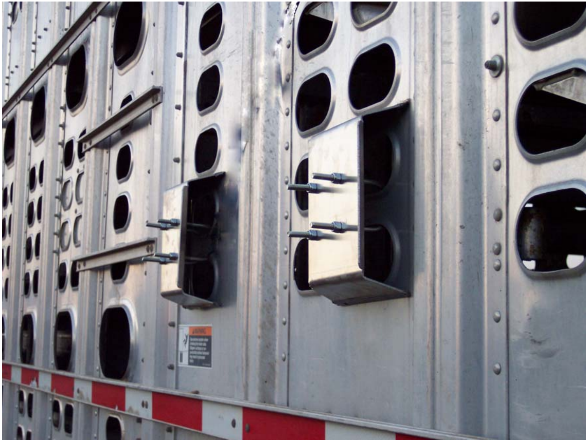
Figure 4. Ventilation scoops secured to the trailer.
