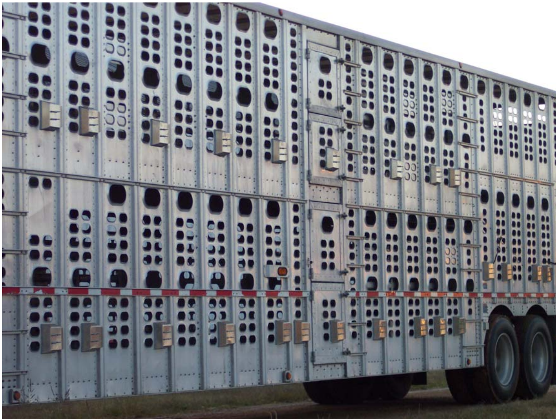
Figure 3. Scoop placement on the ventilated trailer. Scoops were placed on every other panel except when built-in features prevented such spacing. Note scoops are in exhaust orientation.
