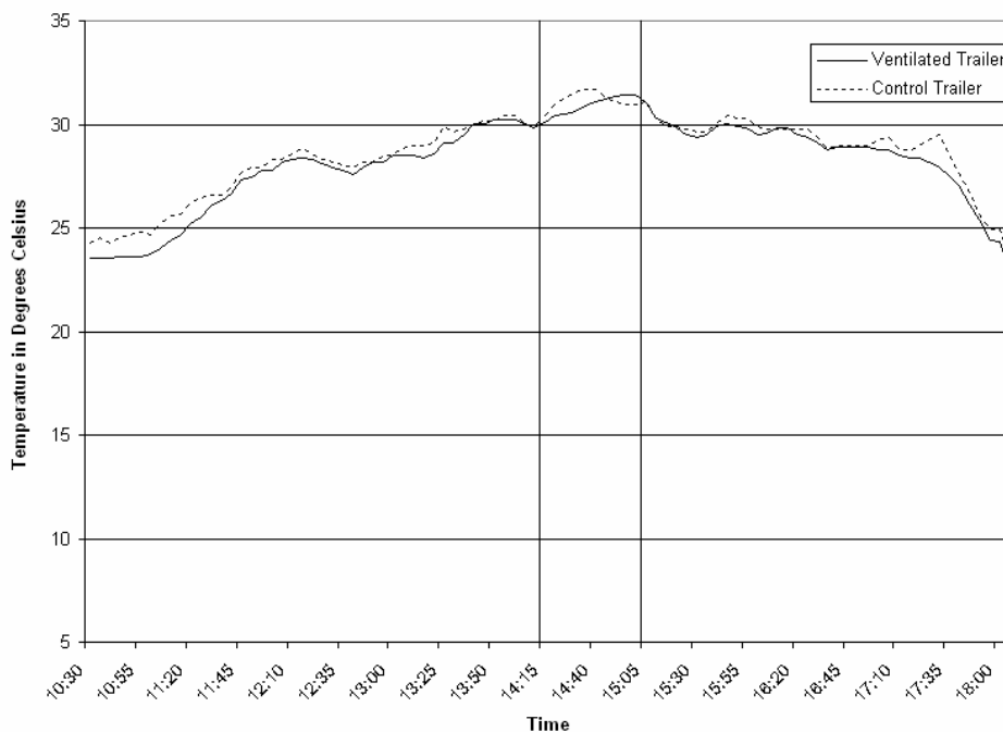
Figure 20. Temperature in degrees Celsius for Trial 2. Temperature was determined by averaging the measurements from all working HOBOs in each trailer. Trailers were parked in the sun from 14:15 to 15:05 during a rest stop, indicated by the vertical lines. Transport continued until 21:30, but temperatures recordings in the control trailer were cut short at 18:05 due to a malfunctioning HOBO.
