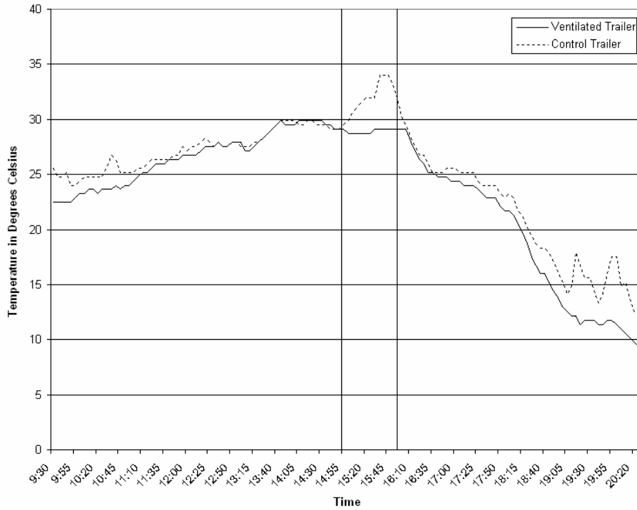
Figure 14. Temperature recorded by the rear HOBOS in Compartment 3 of the ventilated and control trailers for Trial 1. Vertical lines indicate the rest stop.
