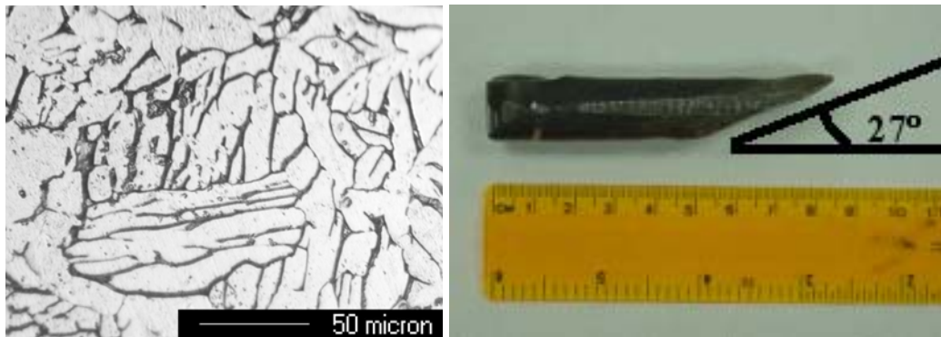
Fig. 5.1. (a) Optical micrograph of as-received Ti64. (b) Extruded Ti64 after a single pass at 800 °C.
