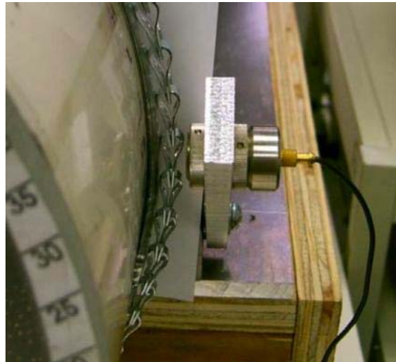
Figure 9: Galvanized chain with magnetic probe.
