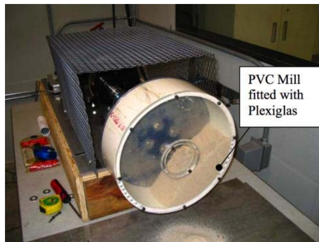
Figure 8: Tumble mill test rig.
