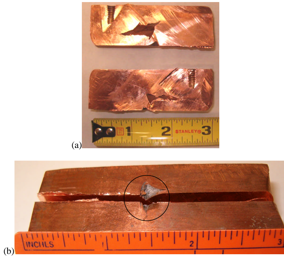
Figure 4.10: (a) Cross section of empty Cu can ECAEd 1 pass at room temperature, and (b) bottom of empty can extruded at ECAE 1 pass at room temperature, showing the bottom indentation.
