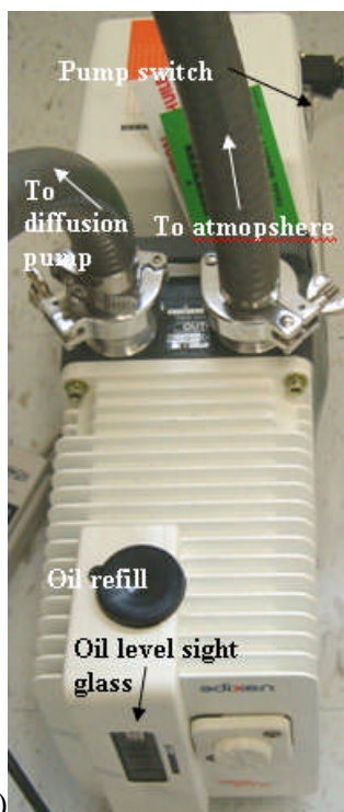
Figure 3.7: The set up of (a) degassing vacuum system, (b) Mechanical vacuum pump, used for degassing and sealing of cans filled with powder, prior to ECAE.
