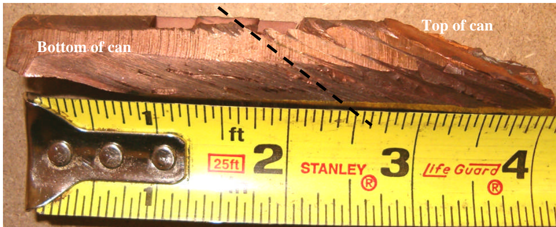
Figure 5.8: Case 22 nc Cu 2B+BP at 100 °C, with back pressure applied after half of the can was extruded. The top of the can half has shear localization, whereas the bottom part of the can is smooth, as a consequence of back pressure.
