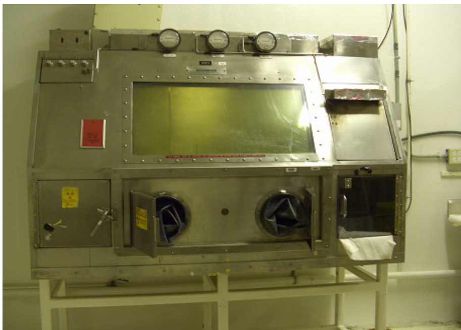
Figure 14 Glove box used to carry out distillation of radioactive iodine.
