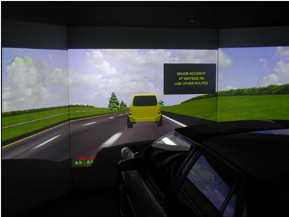
Figure 11. Simulated Highway Scene Presented in TTI’s Driving Simulator
