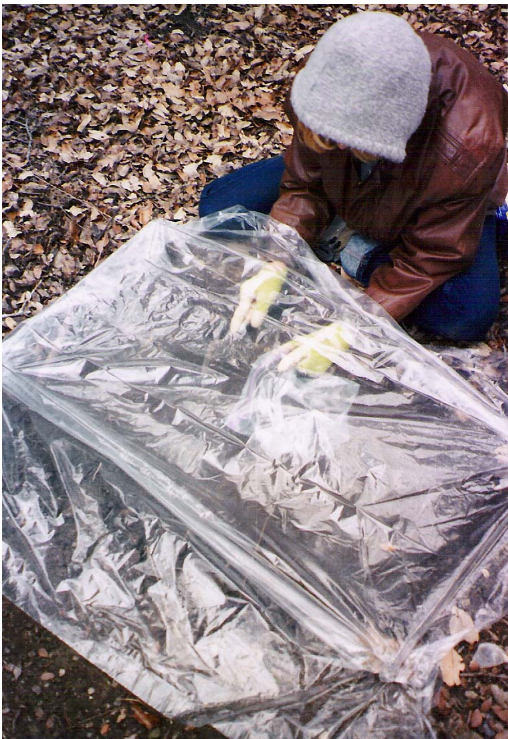
Figure 2.11 Taking Samples at the Rainbow Lake Site Using the Alternative “Mini Tent” Made with Welding Rods.
