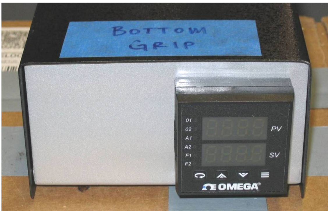
Figure 3.10 Temperature controller used to control thermal management system.
