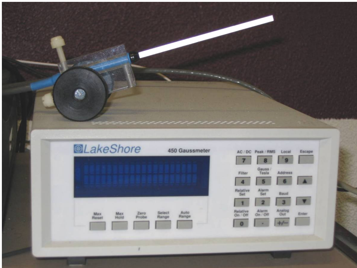
Figure 3.12 LakeShore 450 Gaussmeter and cryogenic transverse Hall Probe used to control electromagnet.
