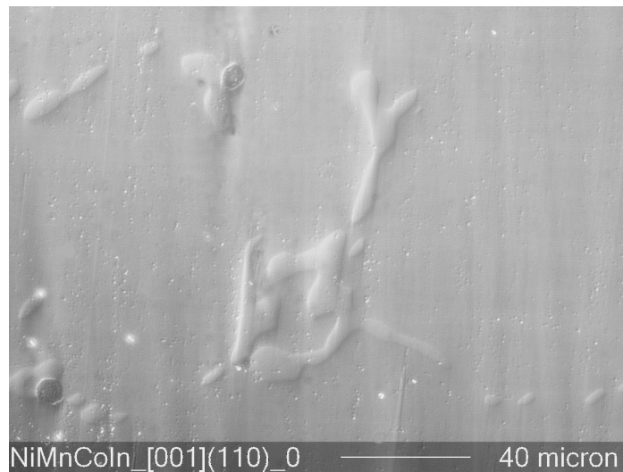
Figure 5.24 Close-up view (20x) of second phase in the NiMnCoIn [100](011) batch 2 single crystal.
