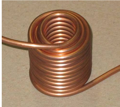
Figure 3.7 Cu coil windings used to channel liquid nitrogen.
