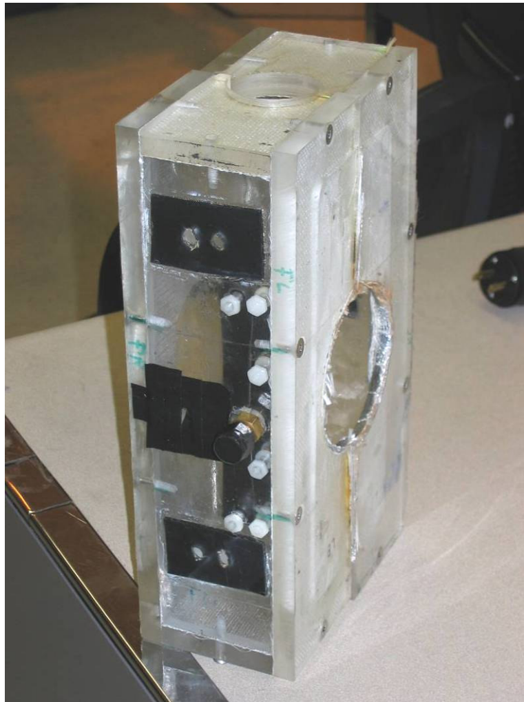
Figure 3.6 Custom lexan box with recess holes for electromagnet pole pieces and compression grips.
