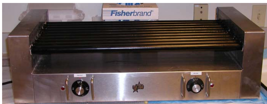
Fig. 11. Hot dog roller used to uniformly coat the scintillation vials with insecticide dilutions.
