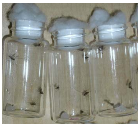
Fig. 12. Insecticide coated vials with five female mosquitoes and a 5x5 mm piece of filter paper soaked in 5% sucrose.
