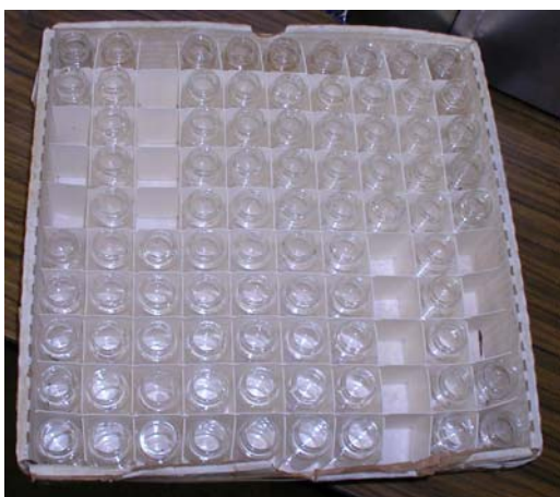
Fig. 9. Insecticide-coated vials for bioassay test.
