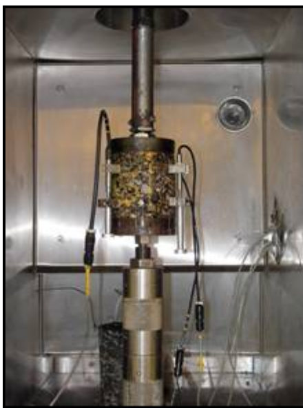
Figure 5.3. Sample setup for the tensile and compressive relaxation tests
