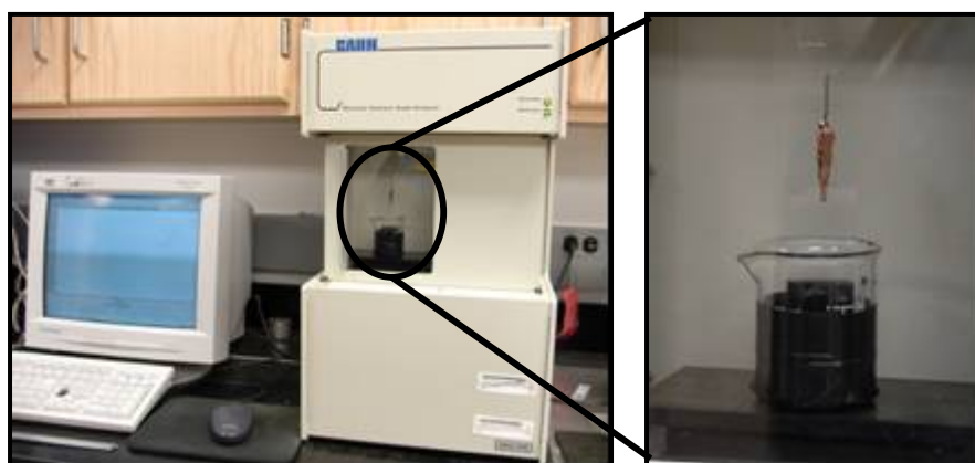
Figure 2.11. Dynamic contact angle analyzer equipment and data acquisition system (left) and sample inside chamber during testing (right)
