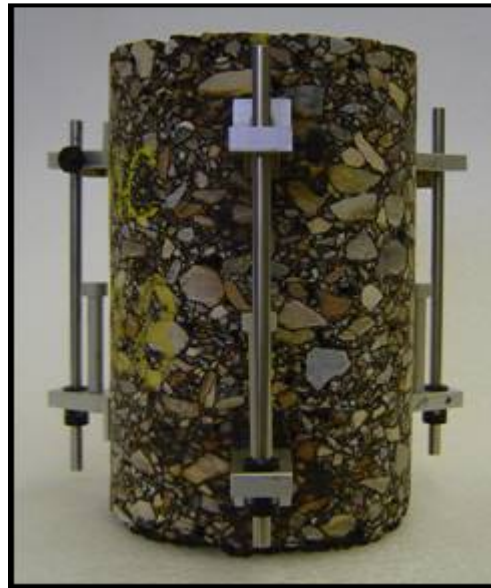
Figure 5.2. Configuration of the LVDT holders
