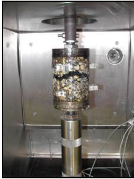
Figure 6.4. Type of sample failure after the completion of the tensile strength test
