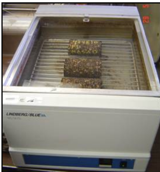
Figure 3.11. Samples submerged in the circulating hot water bath during the moisture conditioning procedure
