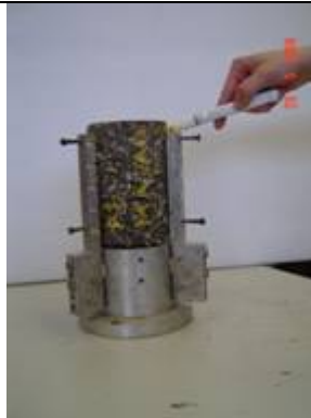
Figure D.1. LVDT Holders' Configuration for the Dynamic Modulus Test
