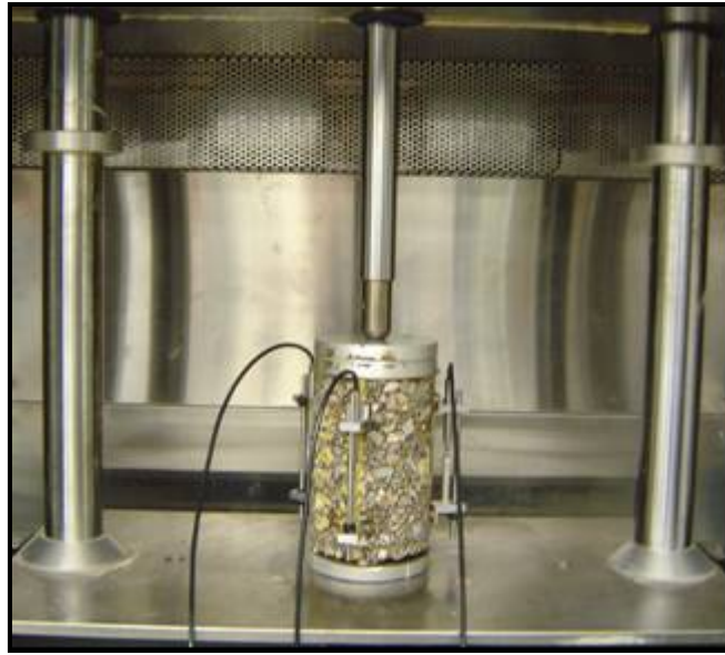
Figure 5.4. Sample setup for the dynamic modulus test inside the environmental chamber of the testing equipment
