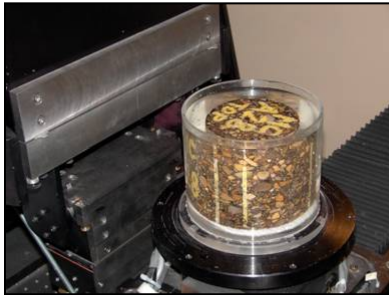
Figure 4.21. Saturated experiment setup during scanning
