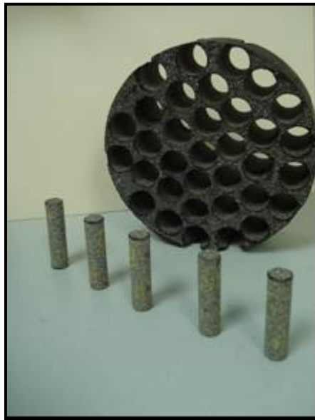
Figure 7.2. Typical asphalt mastic samples used for the DMA test
