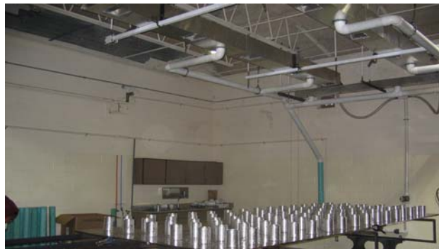
Figure 8. Uniformity distribution testing with 96 aluminum cans
