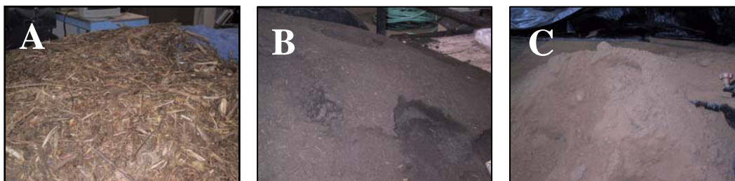
Figure 4. Source materials for treatment (A: untreated woodchips, B: compost, and C: topsoil)
