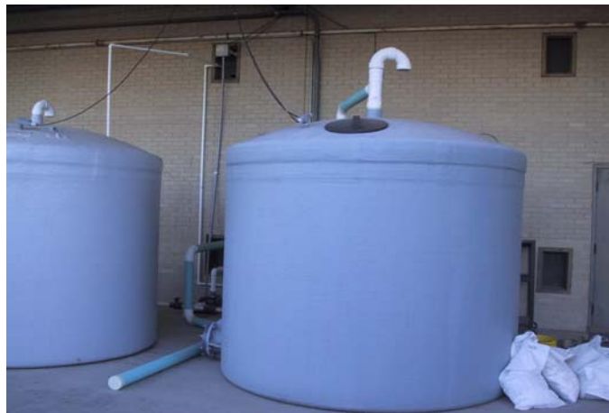
Figure 7. Water storage tank for rainfall simulator
