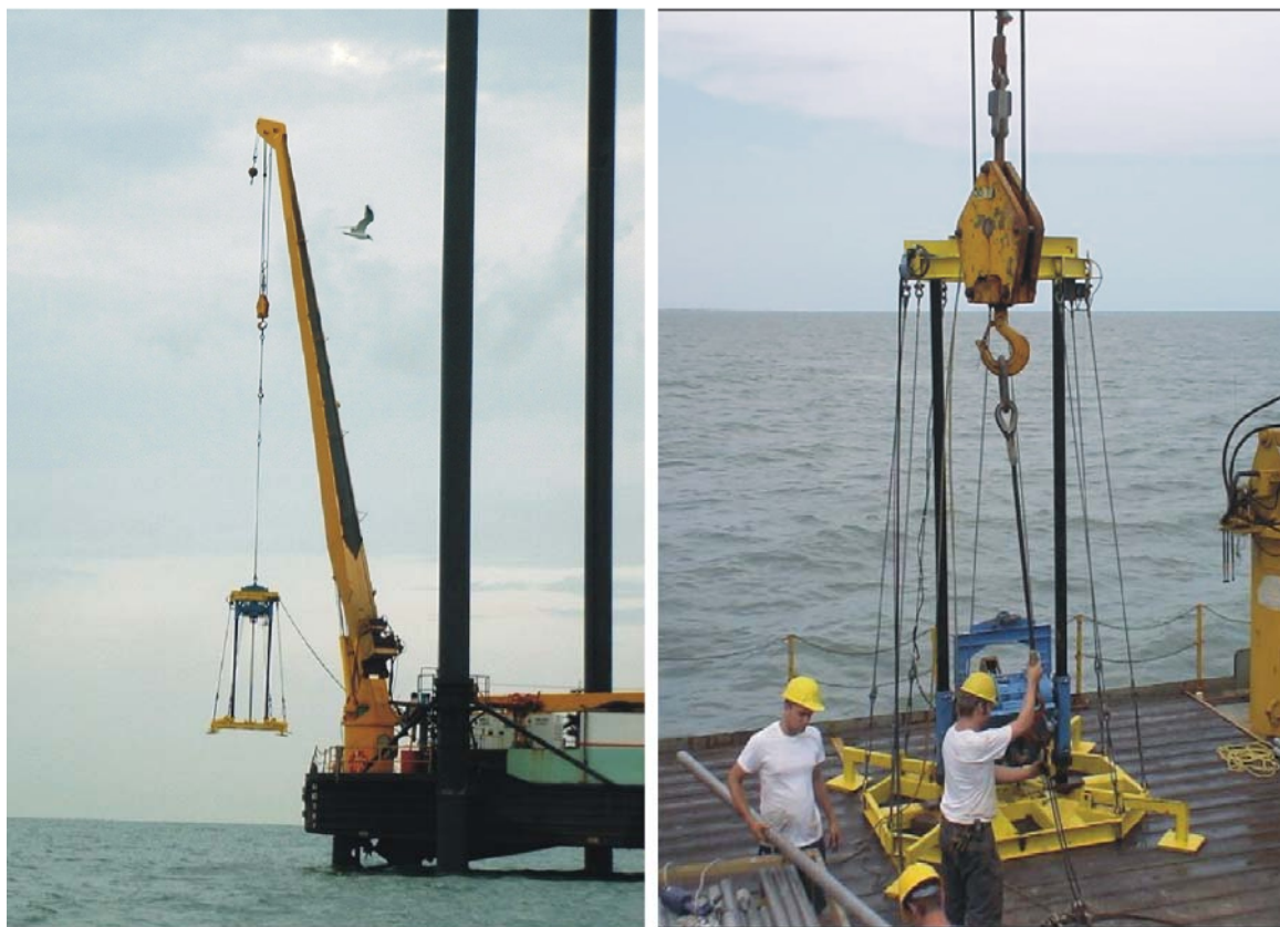
Figure 5: Lift Boat Pontchartrain deploying submersible vibra-core rig for sediment core acquisition (Left). Crew preparing rig with new core barrel before deployment (Right).
