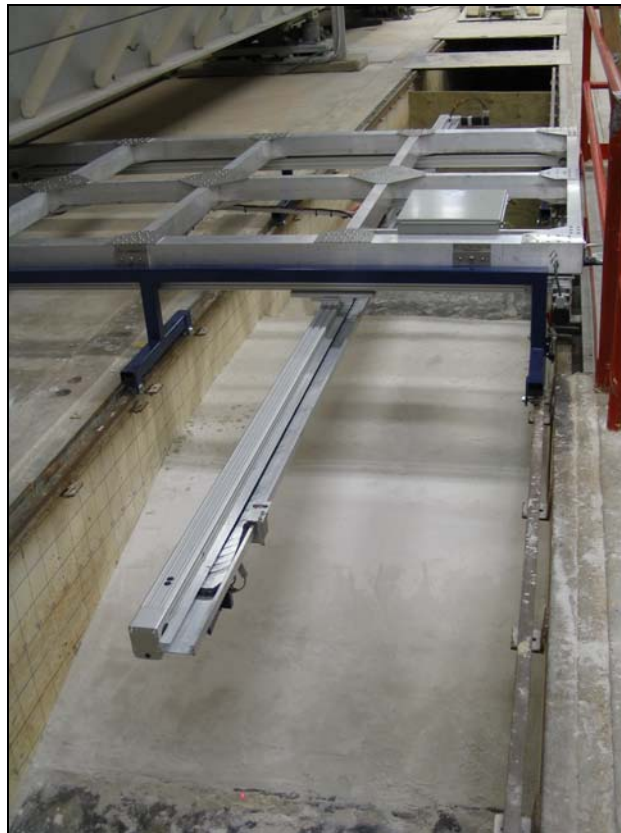
Fig. 4.6. Laser profiler for scanning of sand profile in the experiment.
