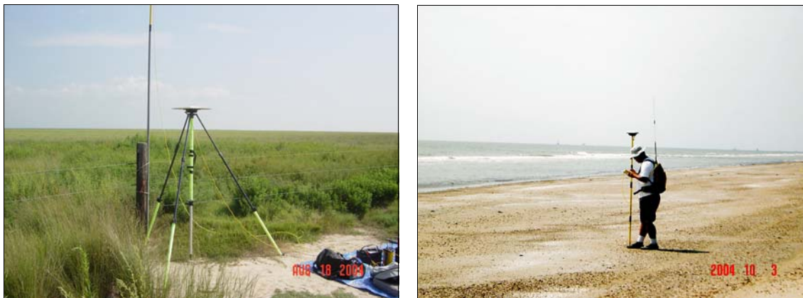
Fig. 3.15. Trimble RTK-DGPS equipment in the survey.
