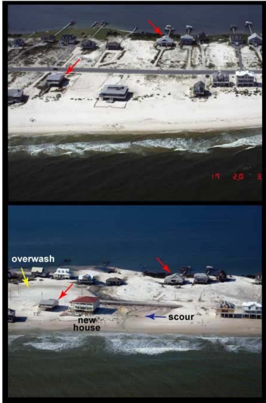
Fig. 2.4. Pre/post storm aerial photography. Overwash across barrier island by hurricane Ivan, Gulf of Mexico, AL (USGS, 2004).
