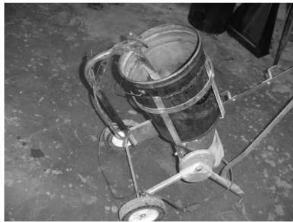
Fig. 3. Mechanical Mixer for Mixing Asphalt with Aggregates.
