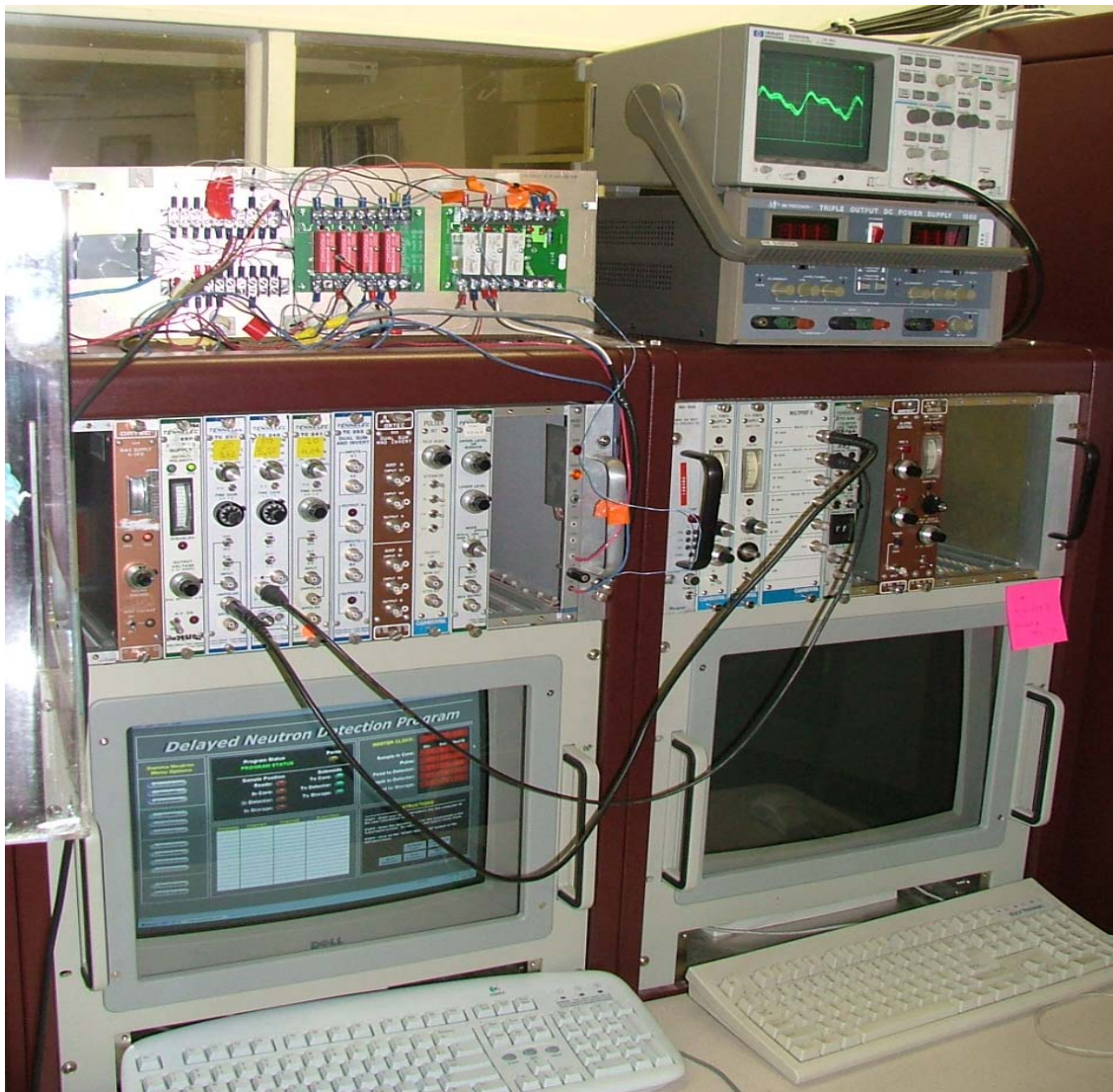
Fig. 14. The electronics and computer control of the counting system.
