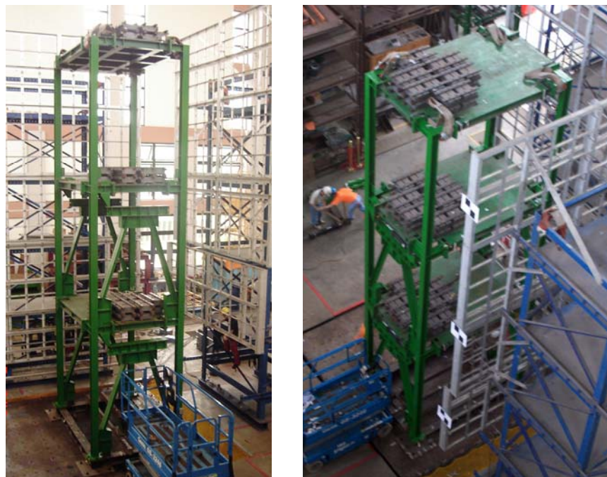
Fig. 98. Torsional Benchmark Structure with Eccentric Masses
