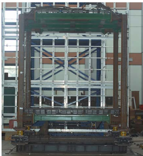
Fig. 99. Base Isolated Benchmark Structure
