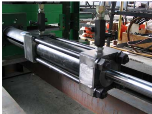
(c) Semi-Active Control Device Fig. 2. Example Control Devices
