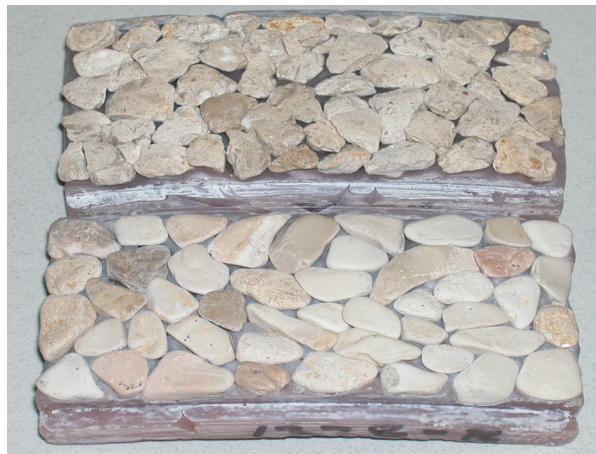
Figure 3.2. Coupon Before and After Polishing.
