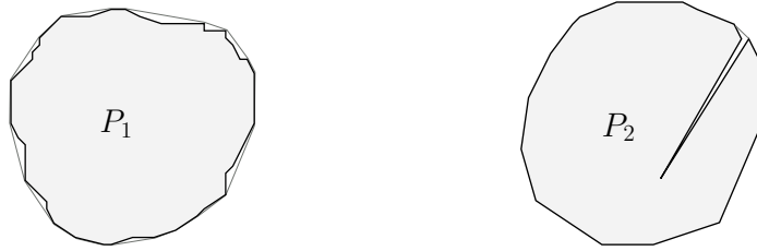
FIGURE 10. Although polygon P_1 is visually closer to being convex than polygon P_2 , this is not identified by their convexity measurements, as defined in Eqn 7.2, which are equal, i.e., \text{convexity}(P_1) = \text{convexity}(P_2) .
