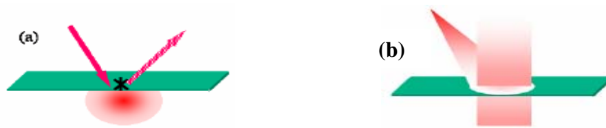
Figure 4 Schematic of different measurement geometries (a) point illumination and point collection and (b) area illumination and area collection geometry.
