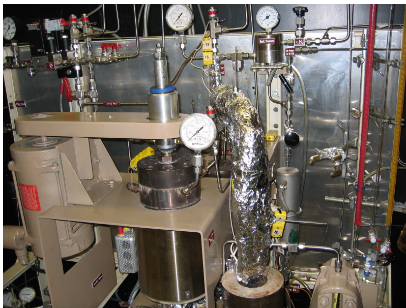
Figure A.3 Robinson-Mahoney reactor assembly. Motor in the left and Agitator on the top.
