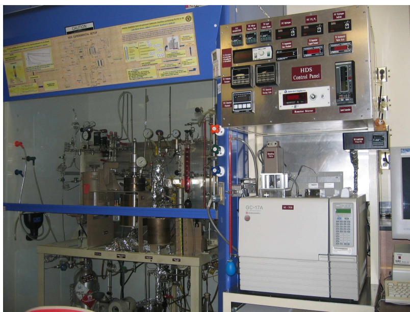
Figure A.5 Control Panel and GC-TCD. Operating variables in the setup were controlled with instruments on this board.
