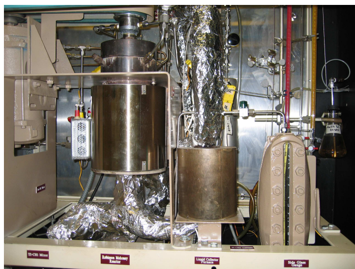
Figure A.2 An experimental Robinson-Mahoney Stationary Basket Reactor used in the HDS of LCO. Front view.
