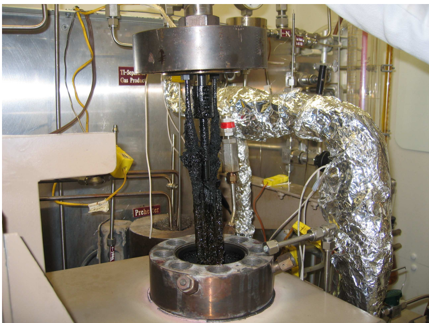
Figure A.7 Coke formed in the HDS of LCO at H_2/HC molar ratio 2.4 or lower (insufficiency of H_2 ).
