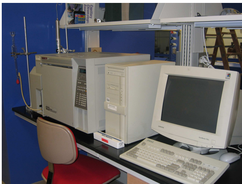
Figure A.6 GCD 1800 Gas chromatograph Mass spectrometer (GC-MS). Equipment used to analyze liquid samples in the HDS of the LCO.
