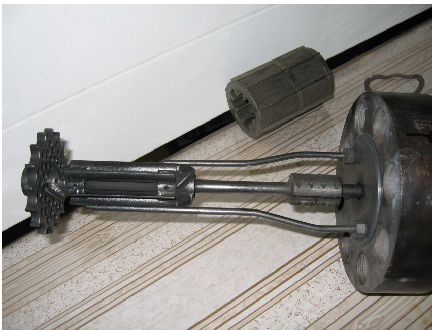
Figure A.7 Coke formed in the HDS of LCO at H_2/HC molar ratio 2.4 or lower (insufficiency of H_2 ).
