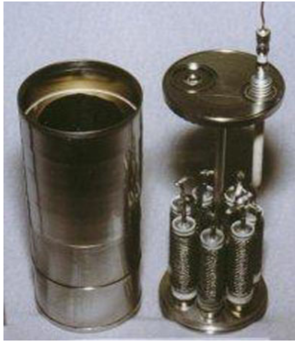
Figure 1.2. Picture of AMTEC cell with 7 BASE tubes.
