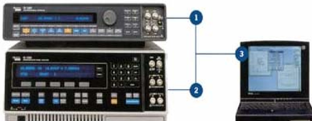
Figure 2.4. Equipment of electrochemical impedance spectrum. 1. electrochemical interface (ECI) 2. frequency response analyzer (FRA) 3. computer and software.
