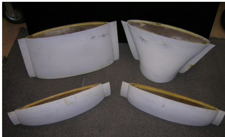
Figure 5: Molds Employed to Create Fiberglass Reproductions of the Inlet Duct
