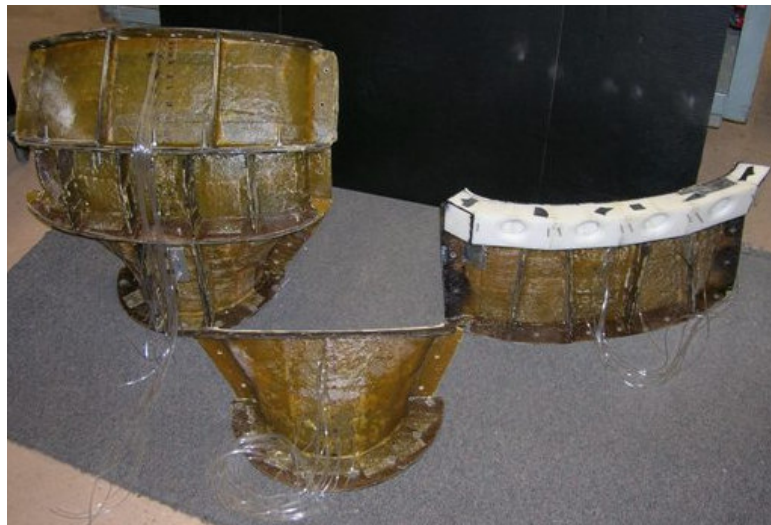
Figure 6: A Set of Fiberglass Duct Sections for the Integration of Flow Control
