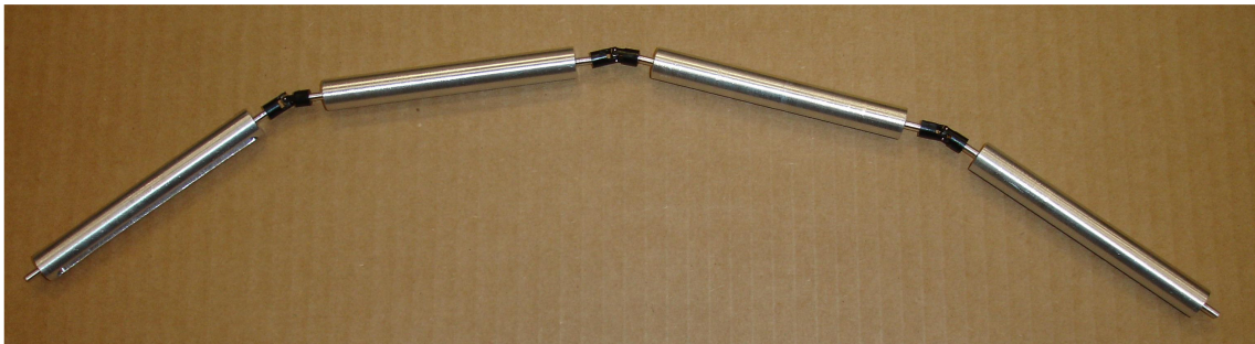
Figure 16: Slotted Shaft Valves Linked with Universal Joints
