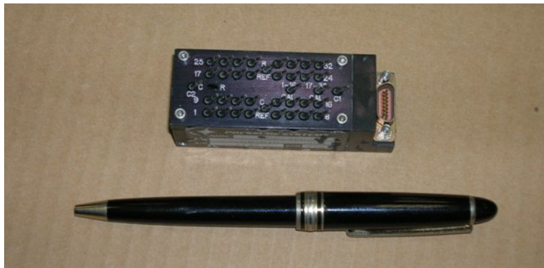
Figure 8: ESP Pressure Scanner for the Rapid Acquisition of Multiple Pressures
