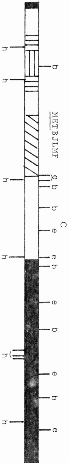
Fig. 7. One possible insertion of the Tn5 element. Letters denote endonuclease cleavage sites: e = EcoRI, h = HindIII, and b = BamHI.
