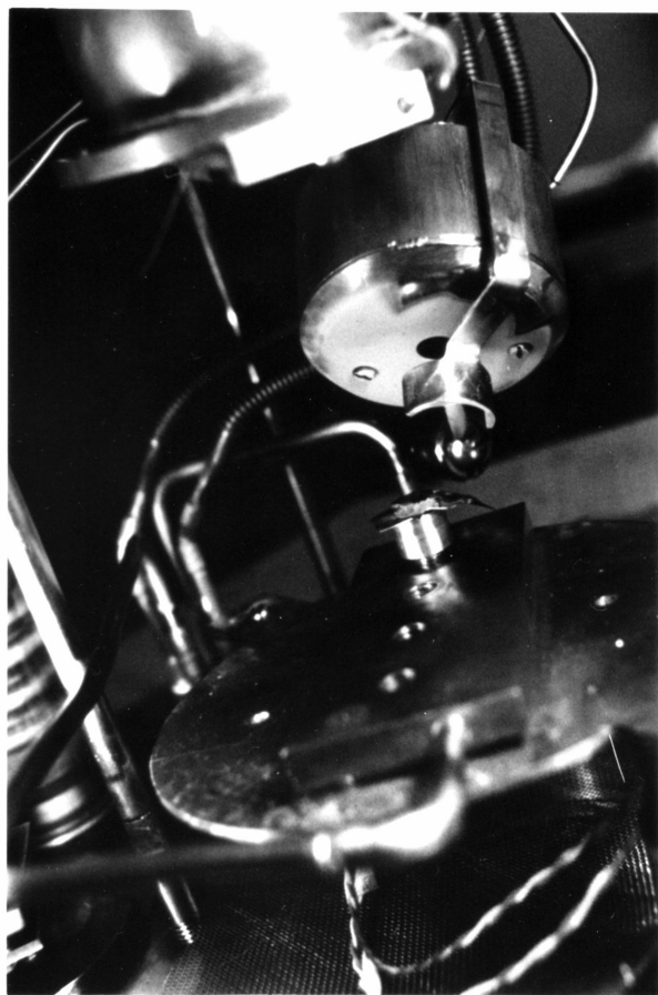
FIG. 10. Two photographs of the electron gun, water cooled target block and crucible, and the substrate holder on the \text{LN}_2 reservoir. The electron aperture in the center of the gun face is clearly seen in the photo on the left. The round crucible is threaded to screw in and out of the holes on the water cooled copper block.
