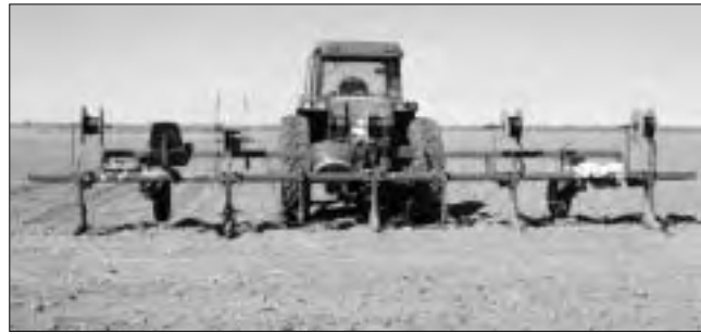
Figure 12. Installation of a subsurface drip irrigation system.
