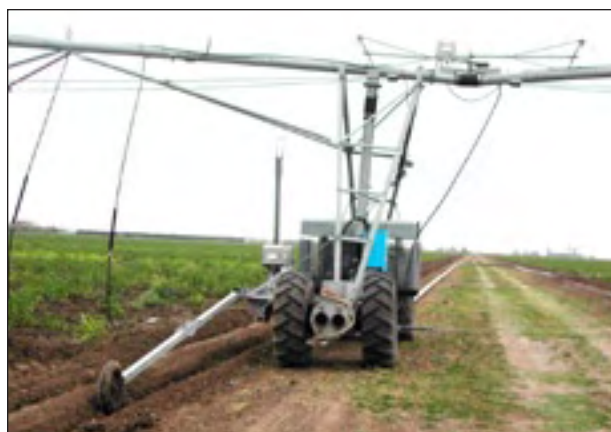
Figure 5. Linear-moving system with water supplied by a hose.
