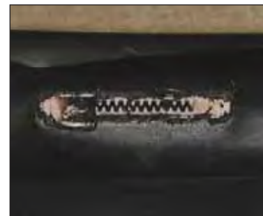
Figure 4. An emitter clogged by manganese oxides.
