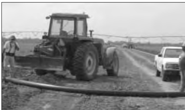
Figure 8. Linear moving system with a flexible hose.
