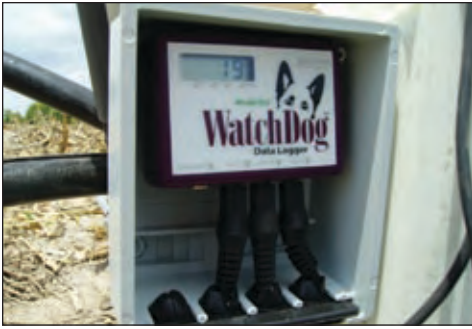
Figure 5. Watermark® sensors connected to a 3-port (up to 3 sensors) WatchDog® data logger.
