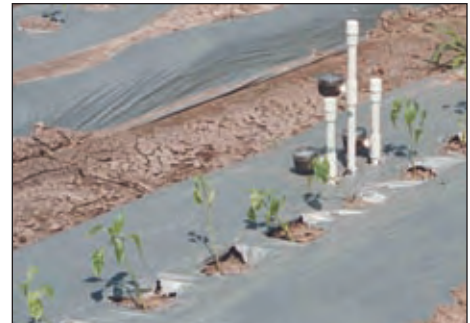
Figure 11. Station of three tensiometers installed at different soil depths.
