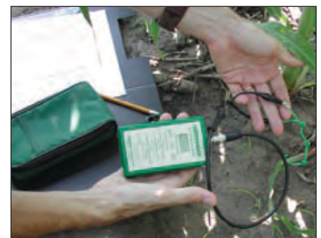
Figure 4. Using handheld meter for Watermark® sensor.
