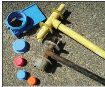
Figure 6. Hole puncher, plugs, and gates for poly-pipe.
