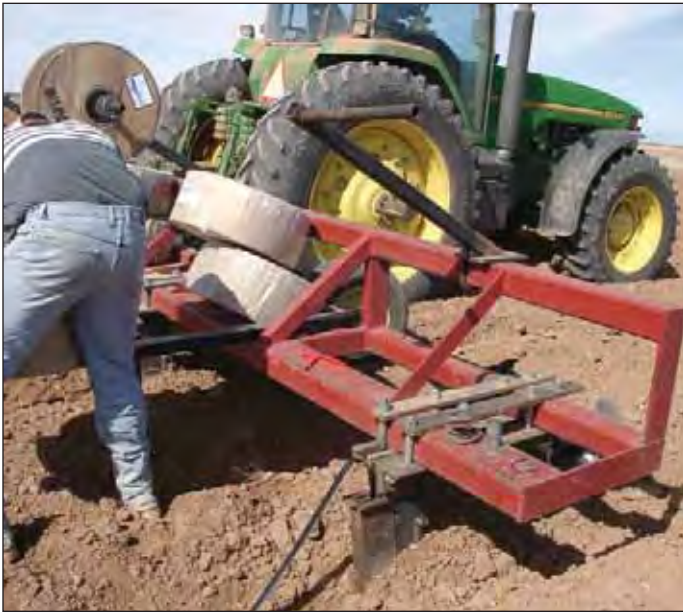
Figure 5. Changing a roll of drip tape in the middle of the field.
