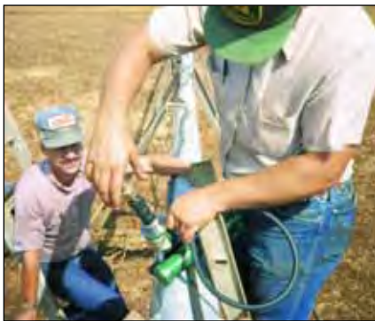
Figure 14. Installing swedge coupler.
