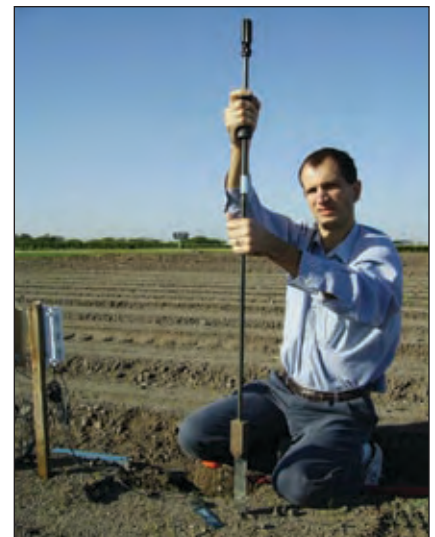
Figure 8. Using a special auger to install the ECH 2 O probes: a blade of the probes shape is hammered down (top) before inserting and pushing down the probe with another tool (below).
