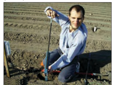
Figure 8. Using a special auger to install the ECH 2 O probes: a blade of the probes shape is hammered down (top) before inserting and pushing down the probe with another tool (below).
