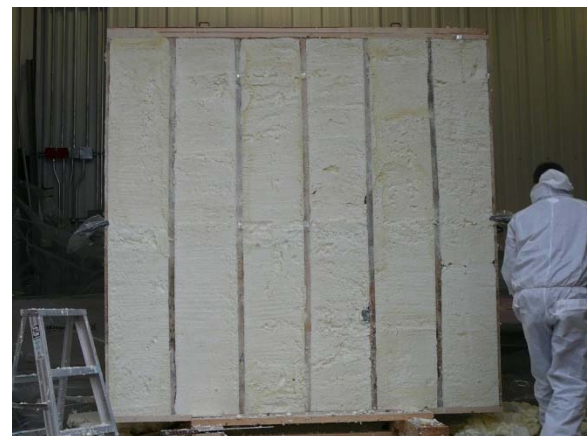
Figure 4 Open cell foamed wall prior to testing.
