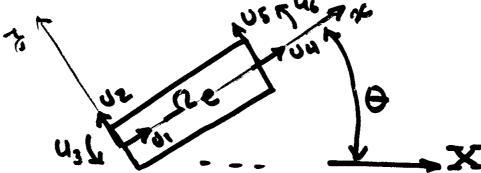
The x-axis is tilted  $\theta$  degrees relative to a <u>global</u> (inertial) coordinate system (X, Y) to which all elements in the structure will be related. In the (X,Y) coordinate system, the displacements are given as:
