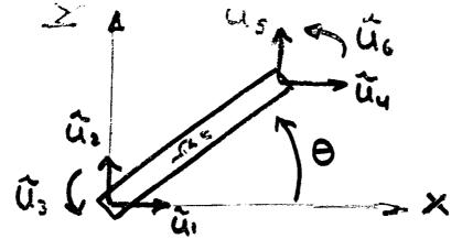
The transformation between the  $\tilde{U}_i$  displacements in (X,Y) to the  $U_i$  displacements in the local coordinate system is given by the transformation equation
