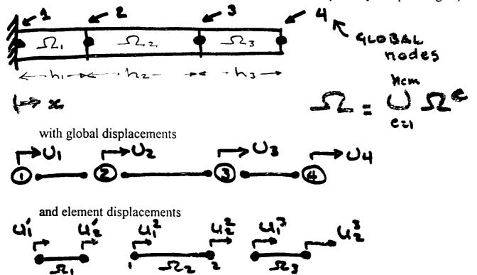
The elements are connected at global nodes (2) and (3) and the displacement u needs to be continuous (i.e., no cracks, fractures, etc.) at these locations, then we must have
