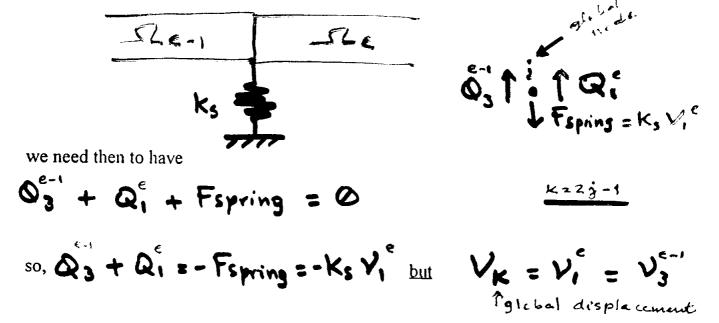
Note that this restoring force depends on the element displacement, and, therefore, it is unknown. At this point, you need to modify the global stiffness matrix and add the contribution of the support stiffness  $k_s$ .
