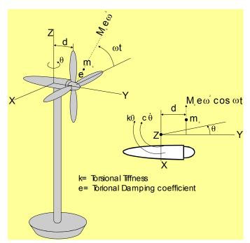
A cantilevered steel pole supports a small wind turbine. The pole torsional stiffness is **K** (N.m/rad) with a rotational damping coefficient **C** (N.m.s/rad).
