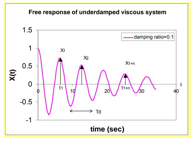
Consider two peak amplitudes, say  $X_1$  and  $X_{1+n}$ , separated by *n* periods of decaying motion. These peaks occur at times,  $t_1$  and
