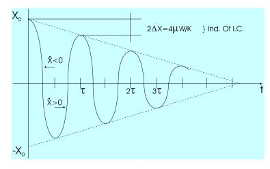
Free response of a mass-spring system with dry-friction
