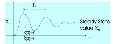
(d) At steady-state, no motion occurs,  $X = X_{ss}$ , and  $\dot{X} = 0$ ,  $\ddot{X} = 0$
