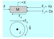
$\begin{aligned} & -\mathbf{F}_{s} = \mathbf{K} \mathbf{x} \\ & -\mathbf{F}_{p} = \mathbf{D} \mathbf{x} \end{aligned} \qquad M \ddot{X} = F - K X - D \dot{X} - F_{G} \quad (1) \\ & I \ddot{\theta} = F_{G} \cdot R \qquad (2) \end{aligned}$
