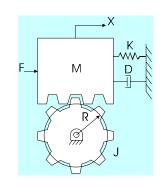
(viscous dissipated energy)  $E_D = \int D \dot{X}^2 dt$ , and External work:  $W = \int F dX$ Derive identical Eqn. of motion (4) from  $\frac{d}{dt} \left(T + V + E_d - W\right) = 0$  (6)
