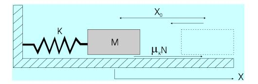
Consider a mass-spring system resting on top of a surface. The kinetic coefficient of dry friction for relative motion between two surfaces is  $\mu$ . Assume that at *t*=0 sec, you release mass *M* from *X*(*0*)=*X*<sub>o</sub>. For a not too large friction coefficient, the mass-spring oscillates about the equilibrium position *X*=*0* with its natural period  $T_n = 2\pi/\omega_n$ .
