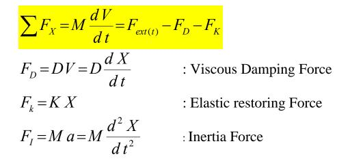
where (M, D, K) represent the equivalent mass, viscous damping coefficient, and stiffness coefficient, respectively.
