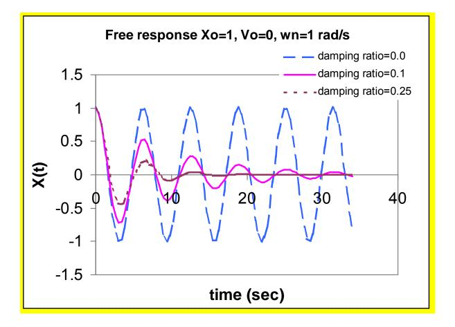
Free Response of Underdamper 2<sup>nd</sup> Order System:Initial velocity onlydamping varies
