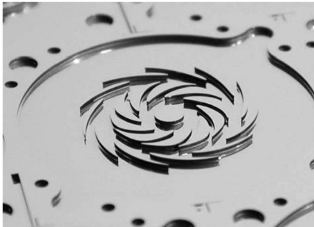
Figure 10: A 500 m/s tip speed, 8 mm dia centrifugal engine compressor.
