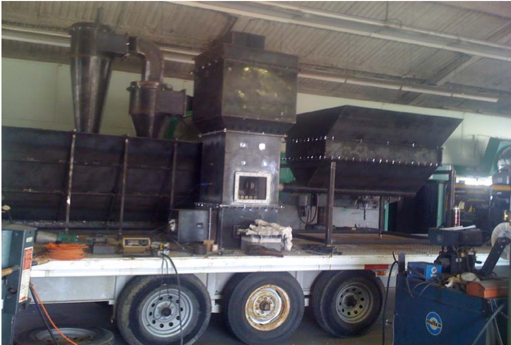
Figure 13. The newly fabricated TAMU fluidized bed gasifier mounted on a trailer.
