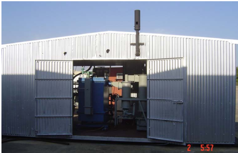
Figure 10. The photo of the TAMU fluidized bed gasifier used in the experiments and mounted on 2.44 m x 6.1 m skid (8 ft x 20 ft).
