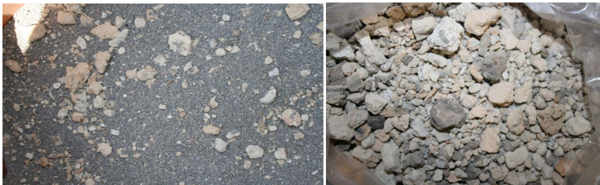
a. Slag formation in reactor
