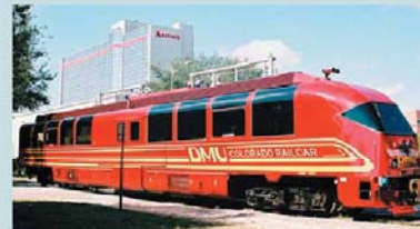
Example of a Diesel Multiple Unit
